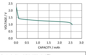
Charging Condition : CV(2.3V, 300 $\Omega$ , 16H, 20°C) Discharging Condition : CR(30k $\Omega$ , 1.0V Cut-off, 20°C)
